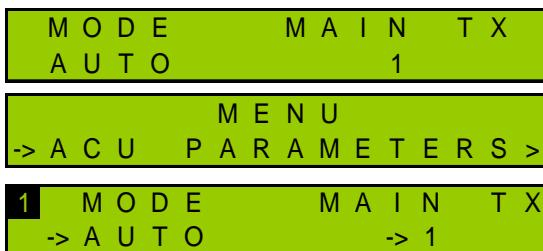
From the main screen, press the "Enter" key to display the ACU Parameters menu.
