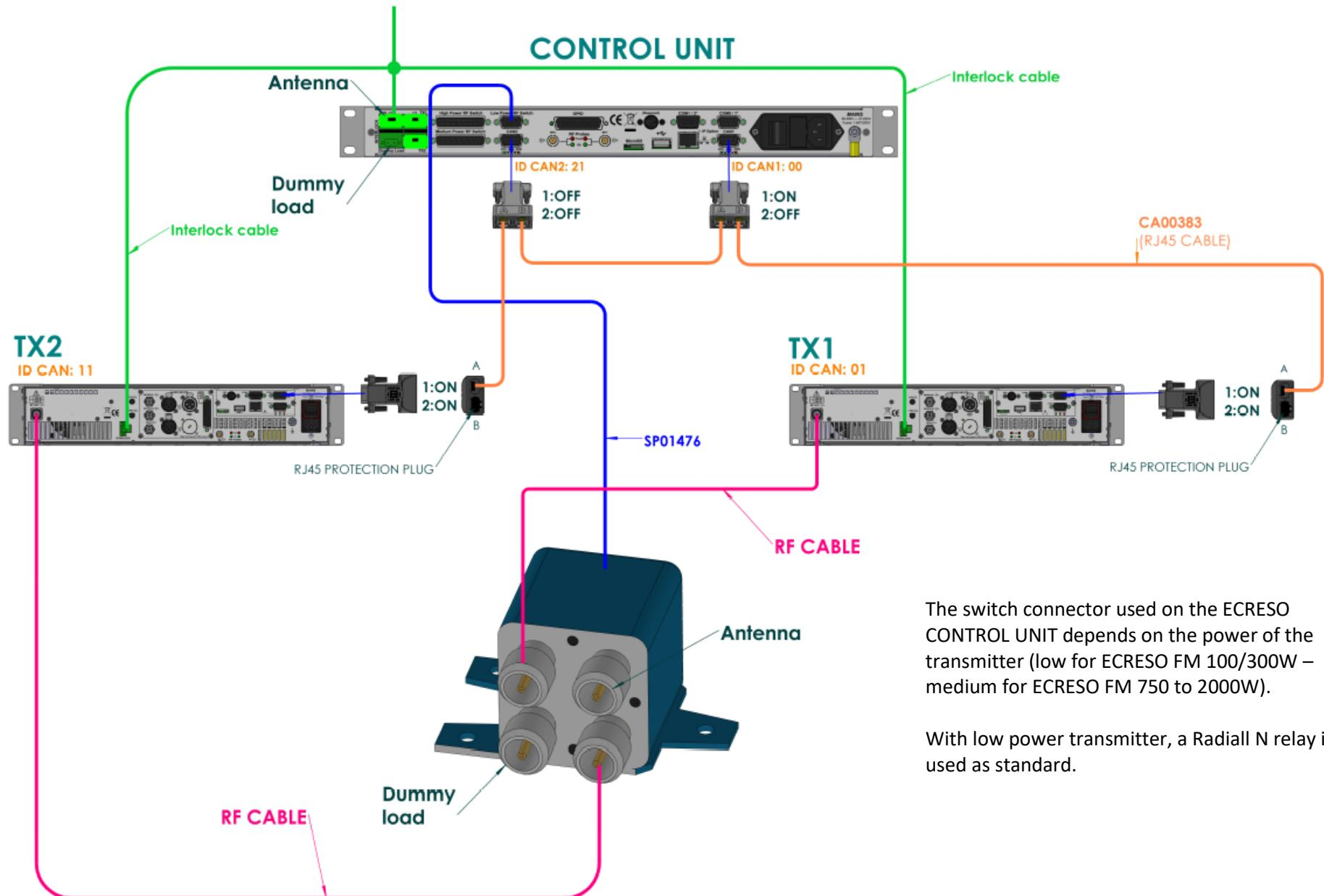
The switch connector used on the ECRESO CONTROL UNIT depends on the power of the transmitter (low for ECRESO FM 100/300W – medium for ECRESO FM 750 to 2000W).
